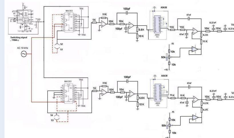
Figure3 : The new conductance circuit design
