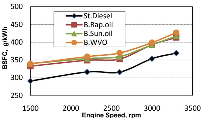
Figure 3: BSFC versus engine speed for fuels tested at full load
