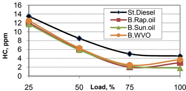
Figure 5: Variation of hydrocarbon emissions with load for fuels tested
