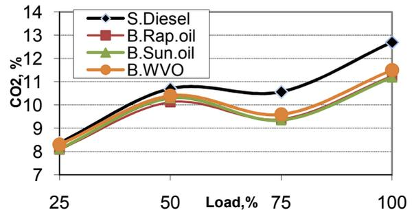
Figure 6: Variation of carbon dioxide emissions with load for fuels tested
