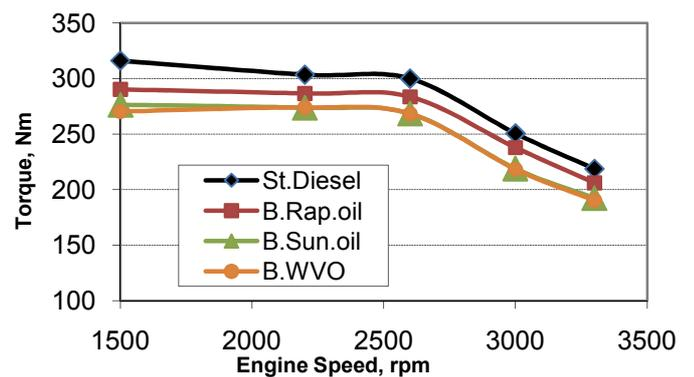
Figure 2: Brake torque versus engine speed for fuels tested at full load
