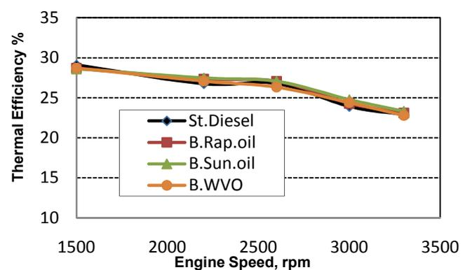
Figure 4: Thermal efficiency versus engine speed for fuels tested at full load
