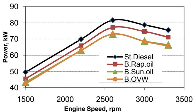
Figure 1: Brake power versus engine speed for fuels tested at full load
