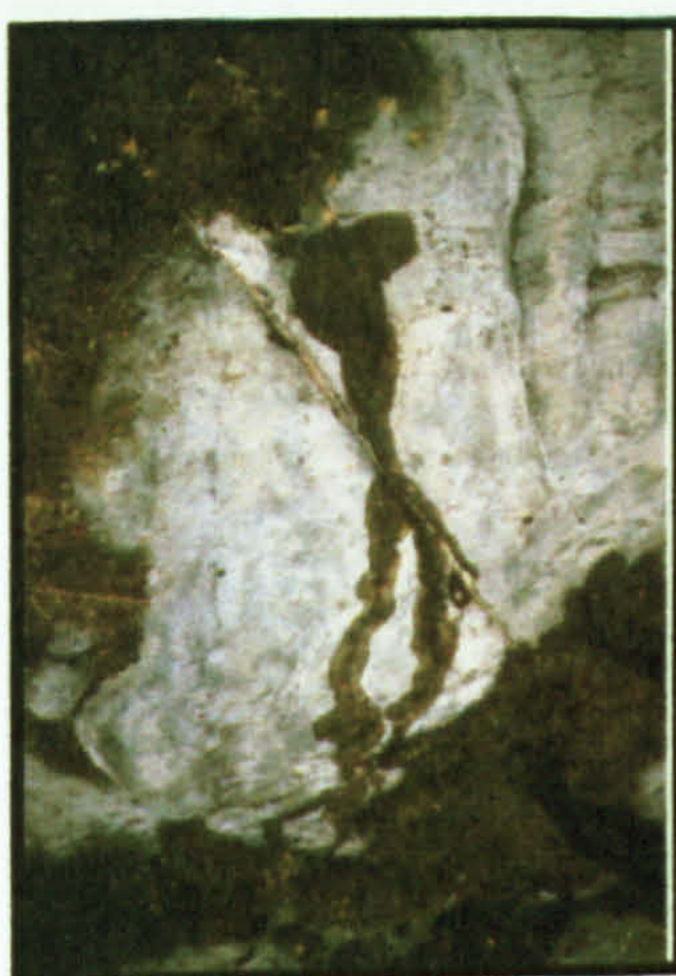
Photo D1.18 Diverging flow Diverging flow of coffee across vertical fracture (Photo 6.16), suggesting that movement occurred after the surface flow had been established.
