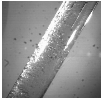
Figure 6: Oil-water inclined pipe flow structure (inclination angle =30 degrees from the vertical Q_w = 3.5 \text{ m}^3/\text{h} , Q_o = 1.0 \text{ m}^3/\text{h} )
