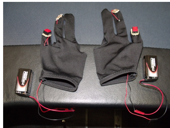
Figures 6.4.3 & 6.4.4: The custom-made gloves that control Screenspat.
