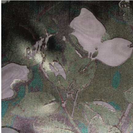
Figure 6: Silk Viscose Satin with devoré and reactive print on reverse of fabric (20)
