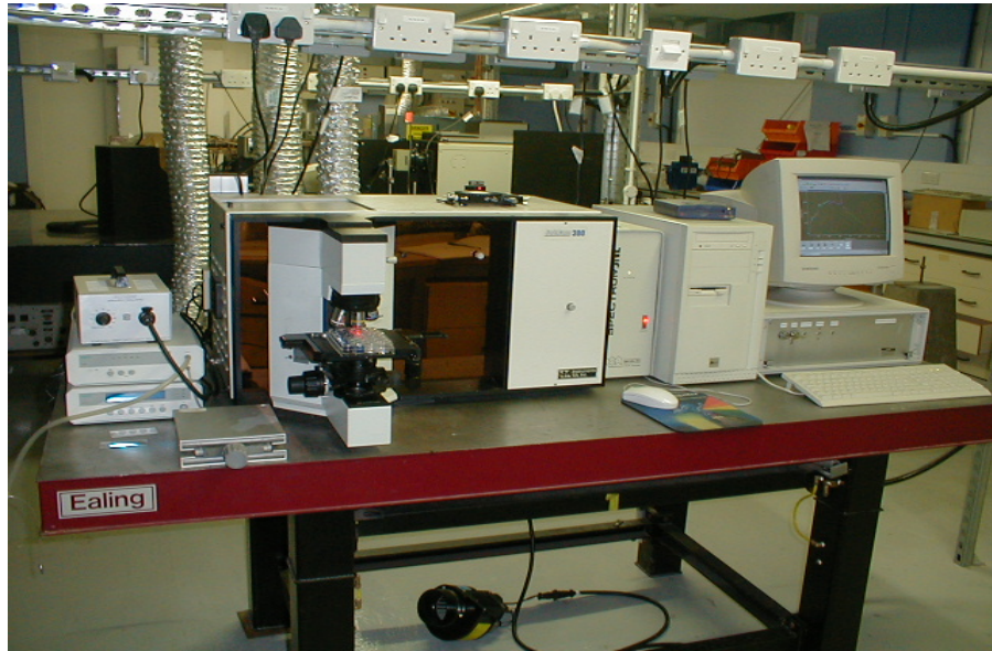
Figure 124: LabRam Raman spectrometer at the University of Greenwich used to conduct Raman experiments.
