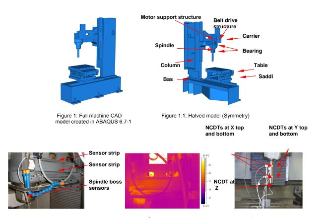
Figure 2: Thermal sensors location machine
