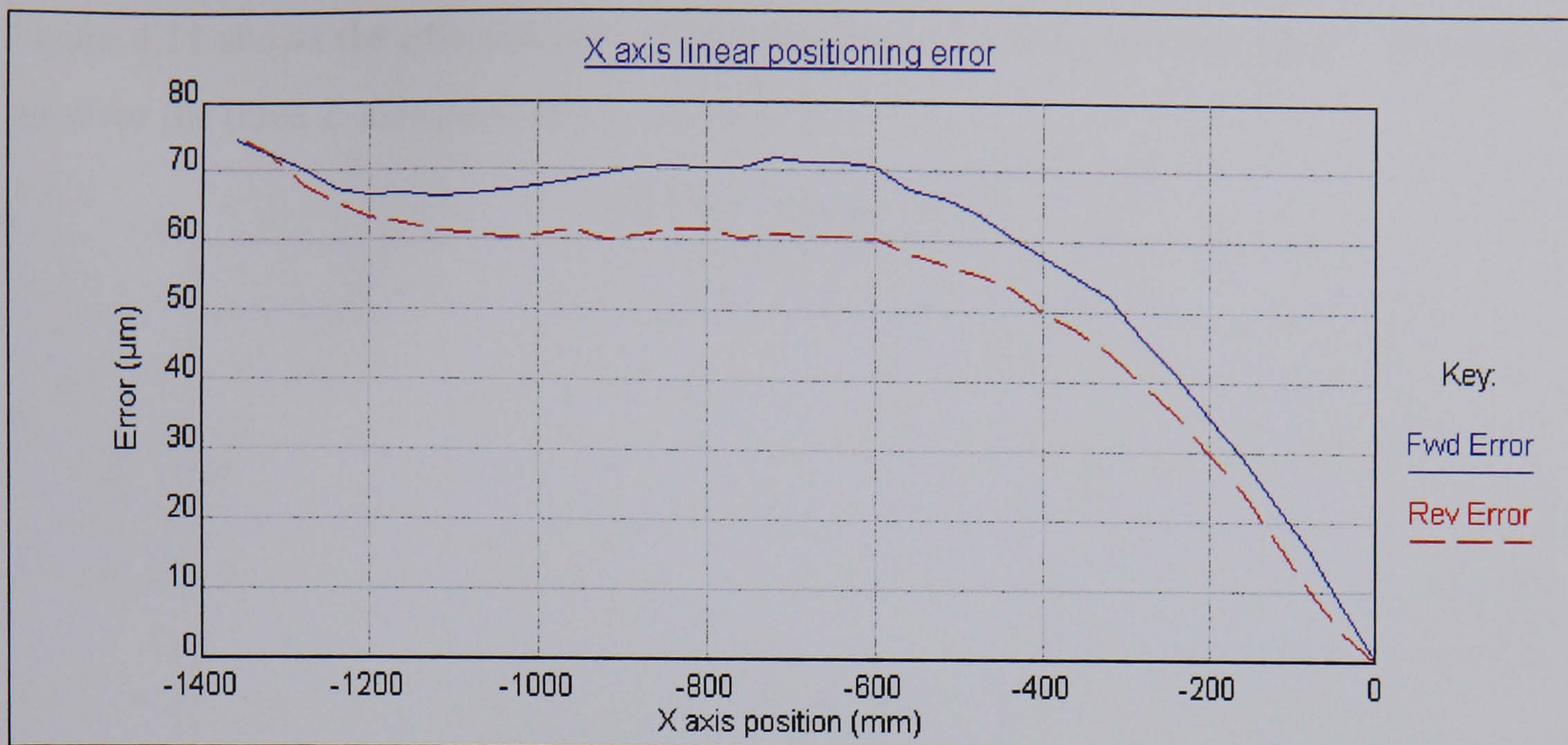
Figure 4.9: X-axis linear positioning error measured with the Z-axis at -800mm
