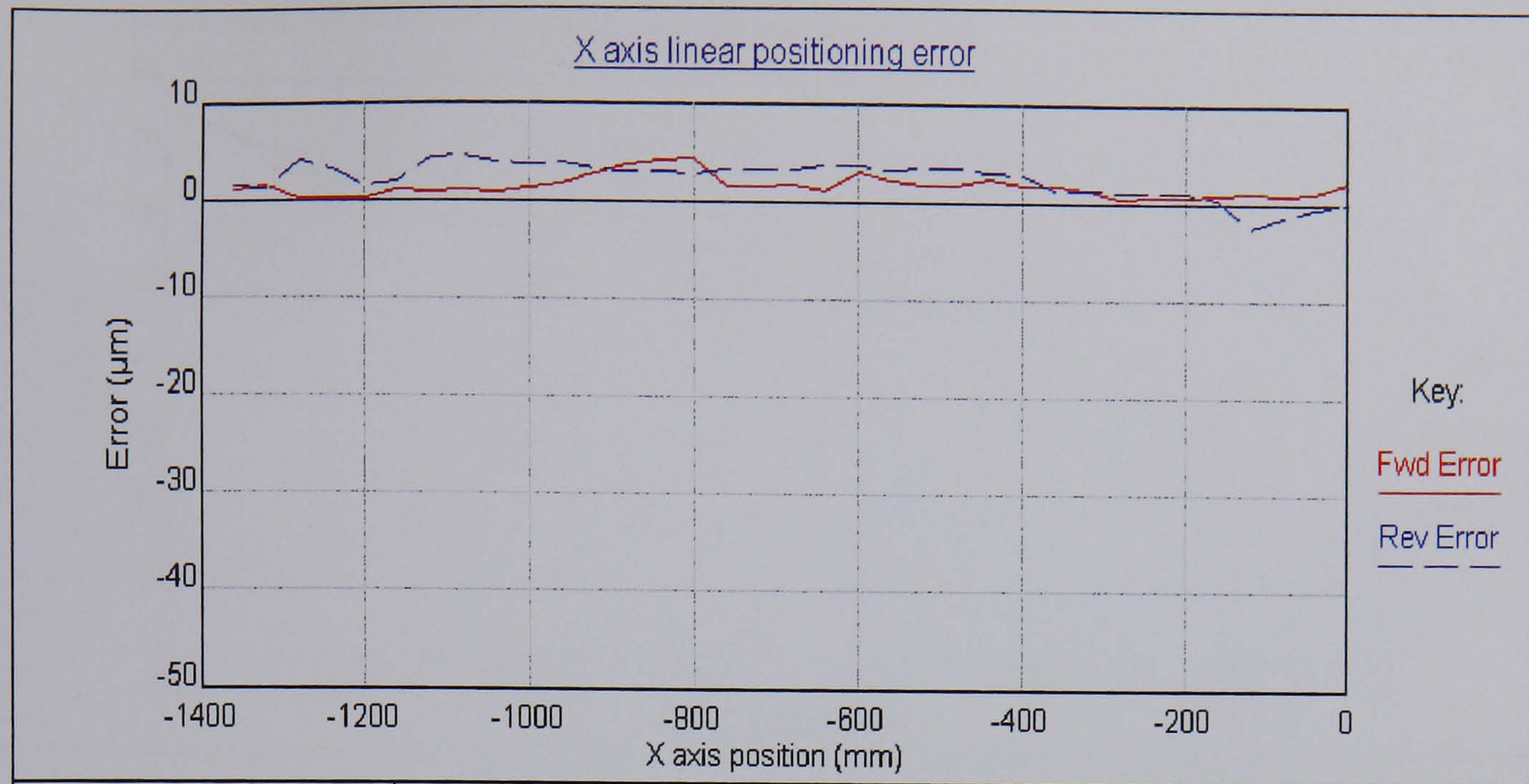
Figure 4.7: X-axis linear positioning error resulting from pitch error after compensation
