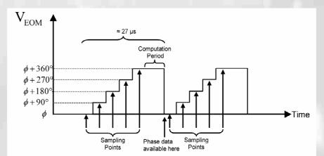
The phase shifting is carried out by applying a stepped waveform to the EOM (see left). After the 5 shifts have carried out, the phase data is calculated by the DSP using the Schwider-Hariharan phase shifting algorithm.
