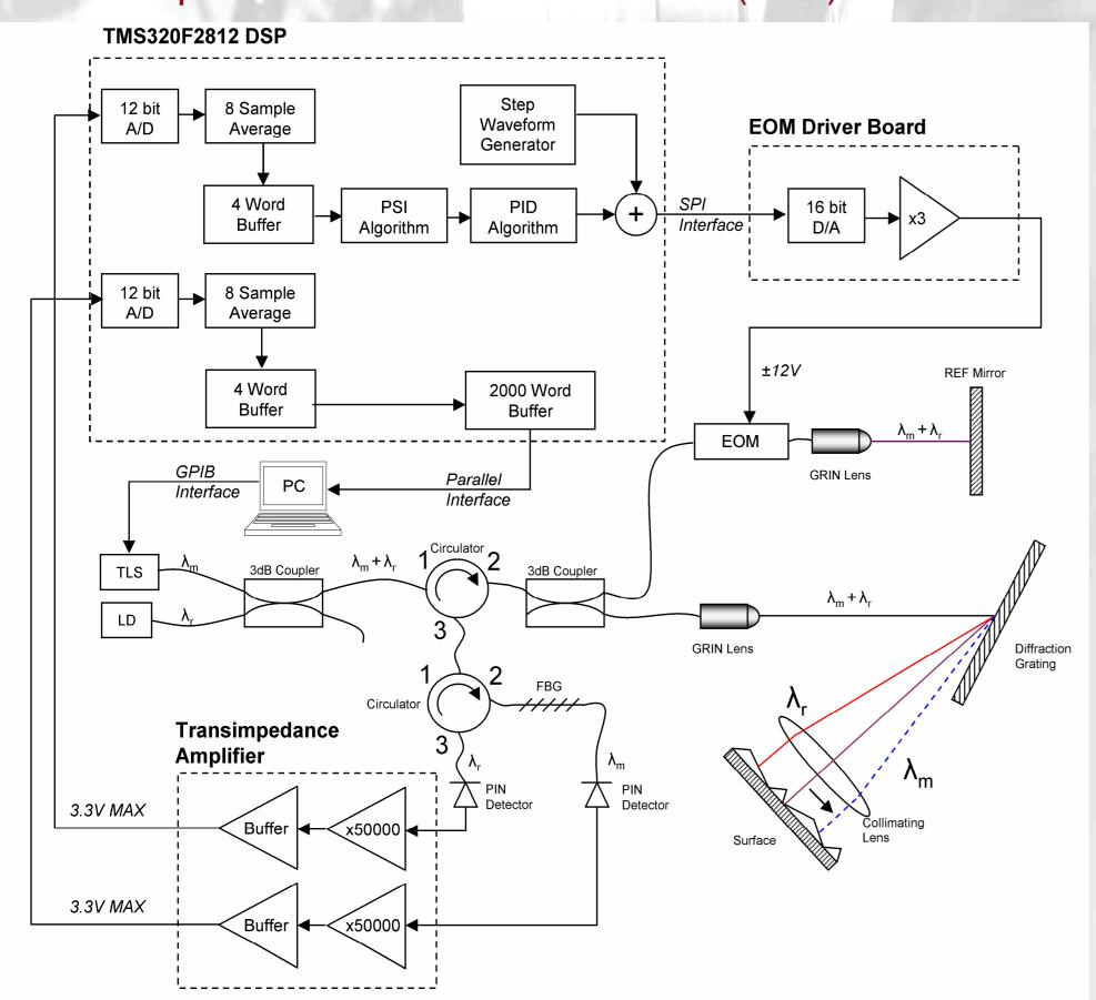
The MFI is comprised of twin interferometers which are multiplexed into an optical fibre and share the same optical path for nearly all of their run. One interferometer runs from a fixed wavelength ( $\lambda_r$ =1550 nm) laser diode (LD) and measures any disturbance due to temperature fluctuation or external vibration.
