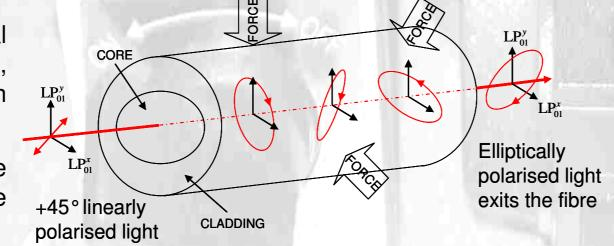
The state of polarisation (SOP) of the light travelling through an optical fibre is constantly evolving as a result of birefringences induced in the core due to strains induced due to deformation of the core resulting from environmental effects. The mechanisms are similar to those which alter the path length.
