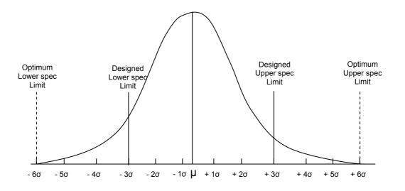
Figure 1 – Normal Distribution, 3 sigma design, 6 sigma optimum design
