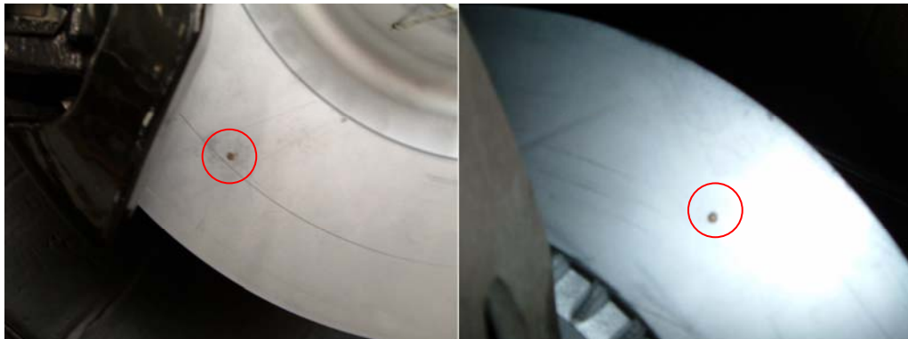
Figure 2: Position of Thermocouples in Front Brake Rotor
