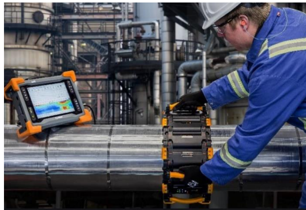
Figure 2-4 Eddyfi lyft (EC) Device used in the field [23]
