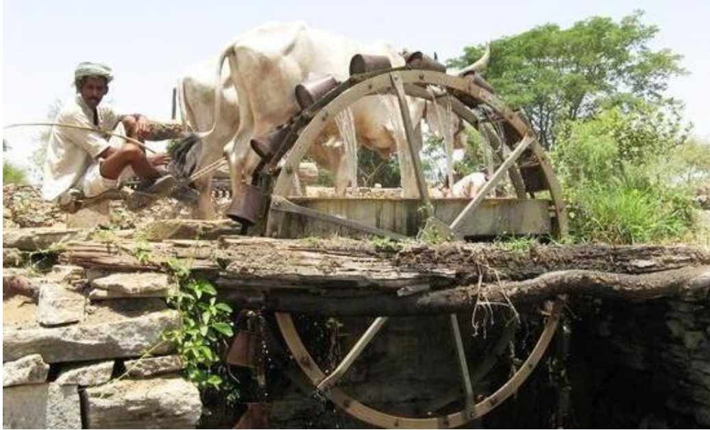
Figure 2- Noria irrigation system (Trevor,2013)
