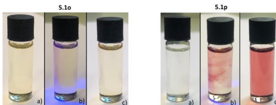
Figure 5.17: Solutions of 5.1o,p in toluene (ca. 1.5 mM); a) before UV-irradiation, b) under continuous UV-irradiation ( \lambda_{\text{max}} 365 nm) and c) immediately after the UV-irradiation ceased
