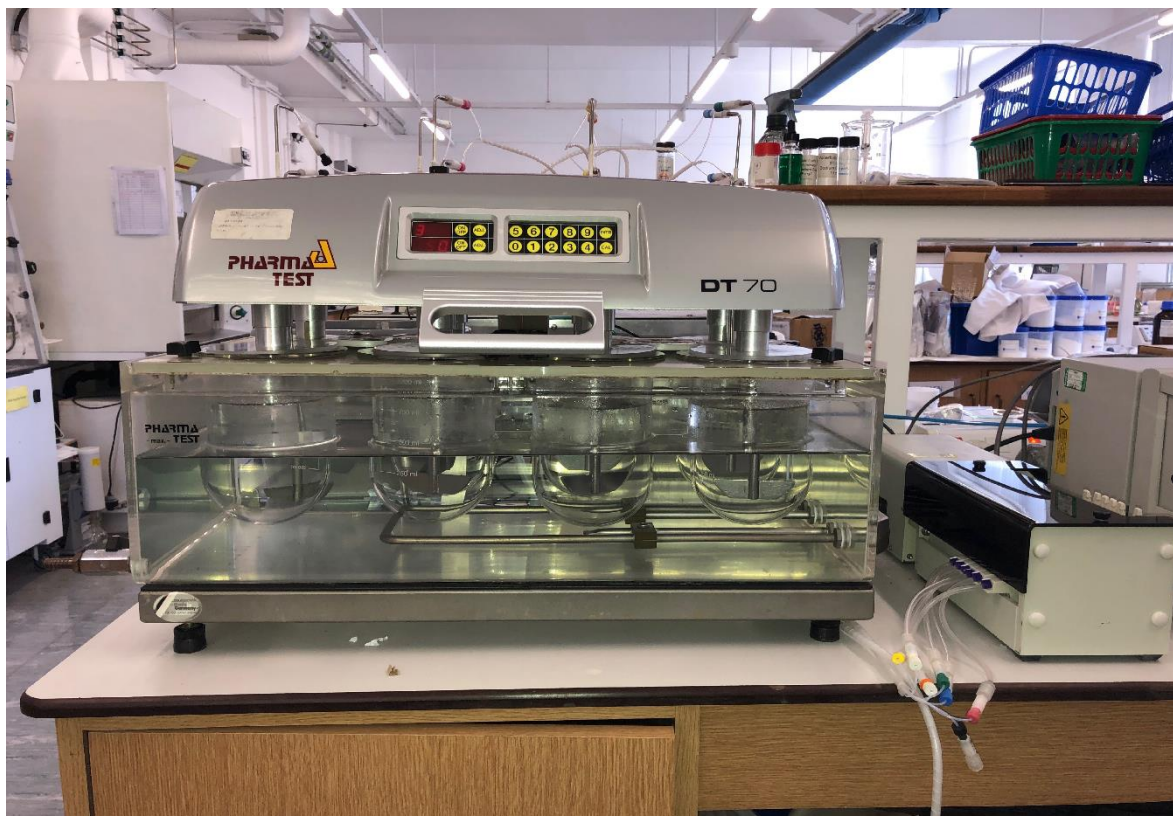
Figure 2. 2. Dissolution apparatus used for analysing formulations.
