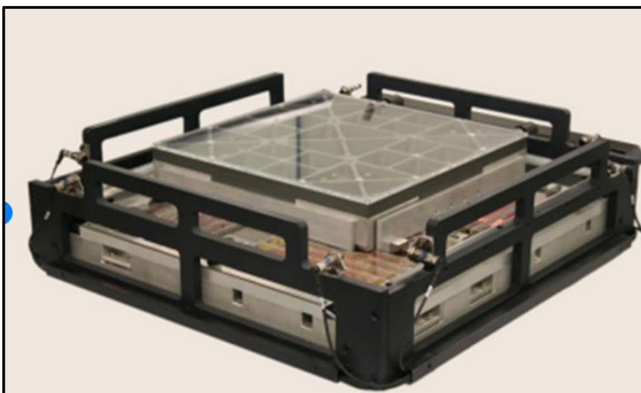
Figure 11 : Shows a planar motor levitated by Tekniker (Altintas, Yusuf & Verl, Alexander & Brecher, C & Uriarte, L & Pritschow, Guenter. (2011)). Machine tool feed drives
