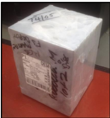
Figure 162 Block of Aluminium 6082T6 square bar (203.2 x 203.2 x 270)
