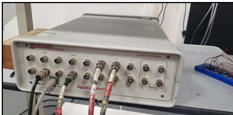
Figure 35A Triaxial accelerometer was connected to data ports of the data box
