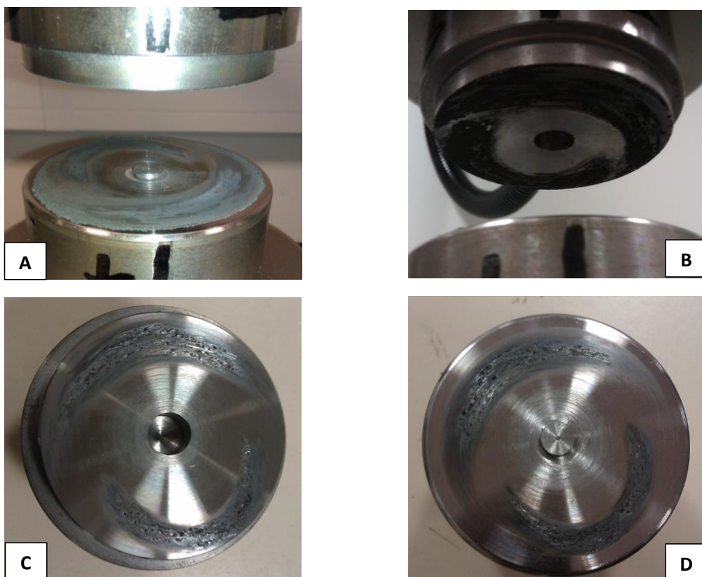
Figure 5.71: (Picture A) Static centre plate. (Picture B) Dynamic centre plate. (Picture C) Dynamic centre plate after the post-test analysis. (Picture D) Static centre plate after the post-test analysis.
