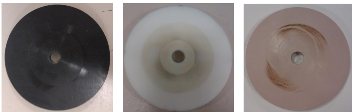
Figure 5.2: Post-test wear liner samples: (Left) Material A, (Middle) Material B, (Right) Material C.
