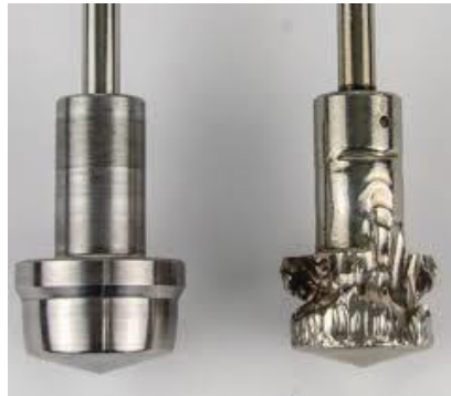
Figure 2.7 Cavitation induced damage to the control valve guide plug [85]
