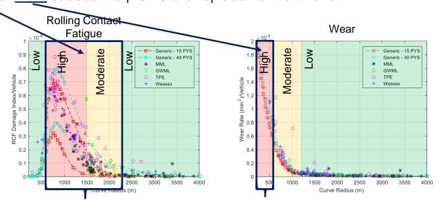
Used in moderate curves to preserve the ground rail profile and increase the resistance to RCF
