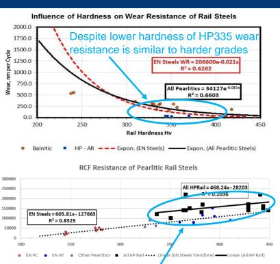
HP rail shows greater RCF resistance than EN grades with equivalent hardness
