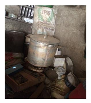
Figure 27: Cooking pot made from salvaged aluminium roofing sheet
