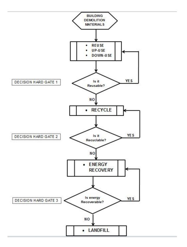
Figure 37: Salvaged Building Materials Handling Process in Kano Nigeria
