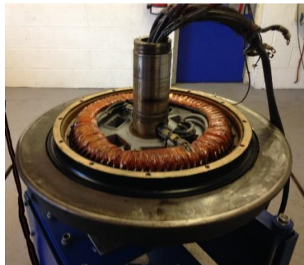
Figure 2: Wheelmotor developed by SET Ltd.
