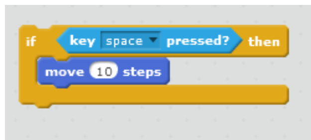
Figure 5: IF statement in Scratch, consisting of 3 blocks
