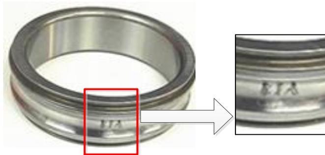
**Figure 7.16 Inner race defect on bearing**
