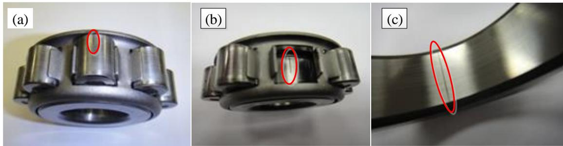
**Figure 6.10 Photographs of fault bearings**
