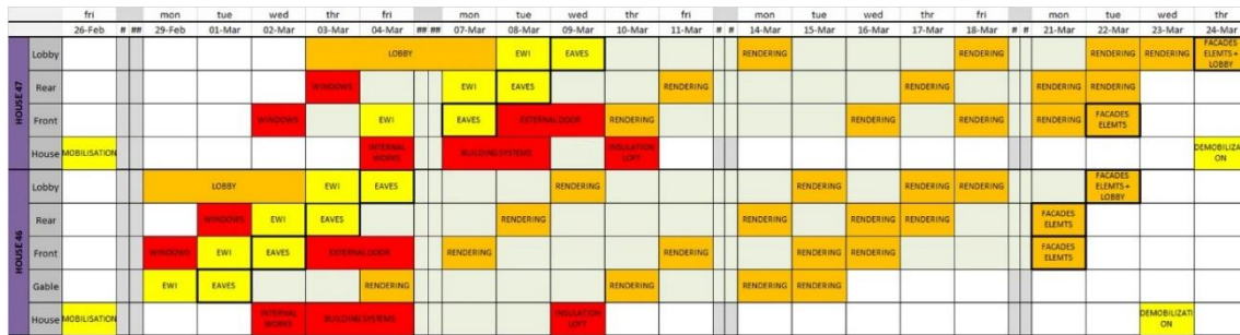
Figure 1. Example of line of balance of scenario 3 with work packages painted according to the end users disruption classification.
