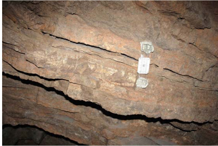
Figure 4: Aperture monitoring using a fissure gauge
