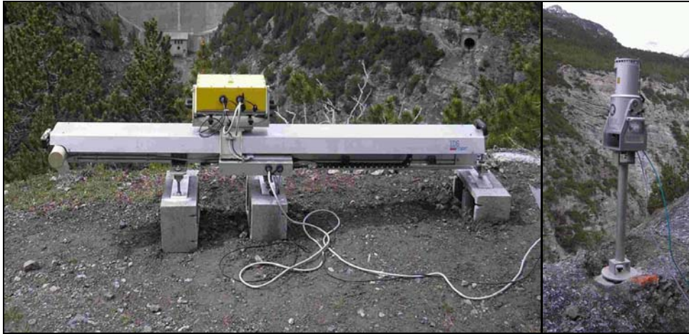
Figure 2: On the left a GB-In SAR system IBIS-L by IDS (Pisa, Italy); on the right a long-range terrestrial laser scanner Riegl LMS-Z429i mounted over a steel pillar for precise repositioning.
