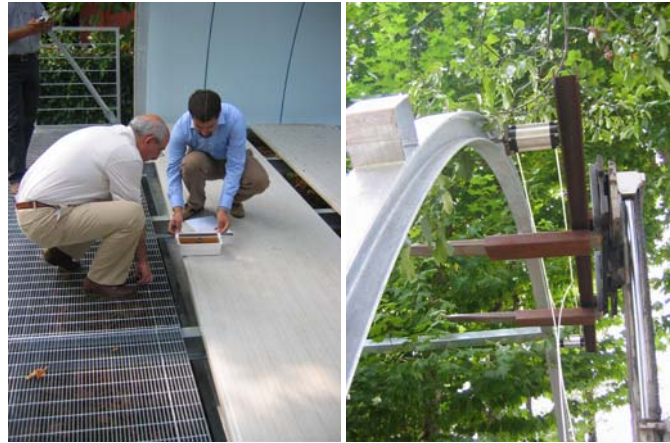
Figures 12 Horizontal load tests have been carried on the prototype by applying hydraulic jacks to the main frames and to the secondary structure.
