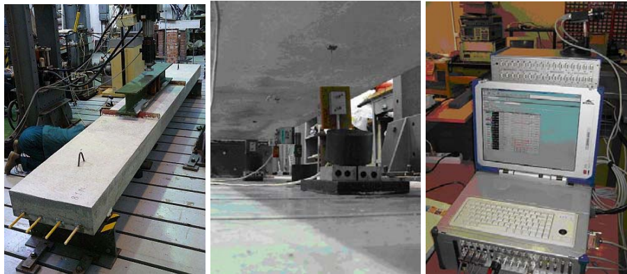
Figure 1. Experimental layout (concrete slab with GFRP - sensors underneath - measuring station)
