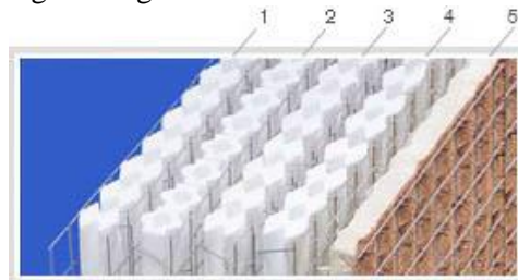
Figure 4 W Panels (core and sheets (5), bars (1, 2, 3, and 4) and grid (Source: http://www.panelw.com/english/index.html )
