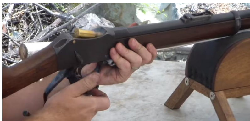
Figure 12. The reality of the cartridge ejection. It was not uncommon for Martini-Henrys to eject quite weakly.
