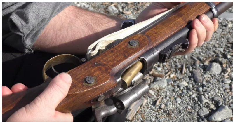
Figure 6. Ejecting the spent cartridge from a Snider-Enfield. 90
