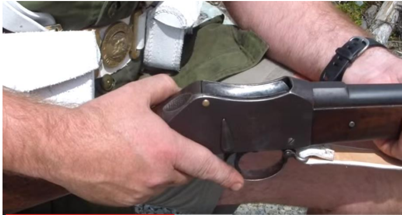
Figure 5. The soldier in the ready position with an un-cocked rifle. Notice that the cocking indicator sits vertically. 207
