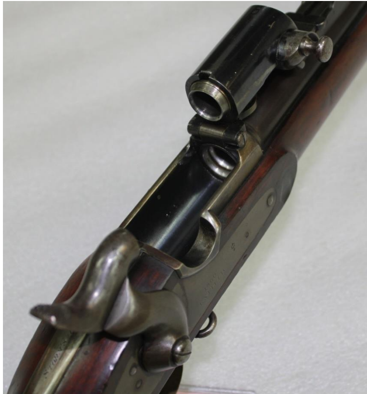
Figure 5. Sealed Pattern Montgomery Storm rifle with open breech. 62
