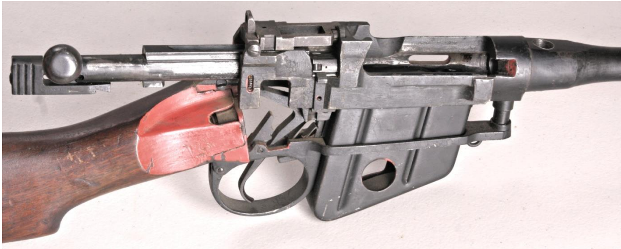
Figure 12. Skeletonised Lee-Enfield showing the open bolt, with the visible cocking piece to the left. 360
