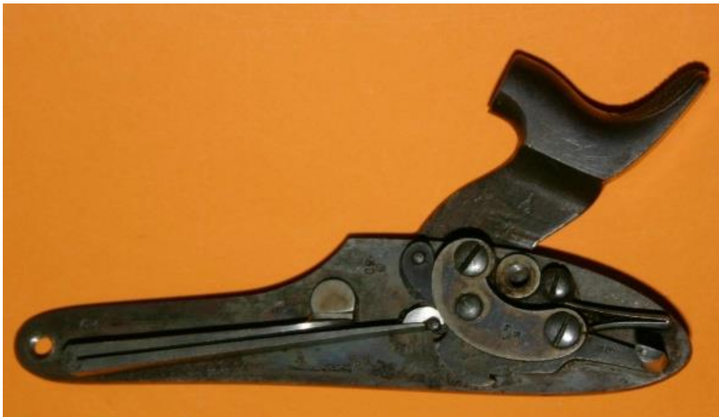
Figure 12. Mk III Snider-Enfield lock at full cock. 96
