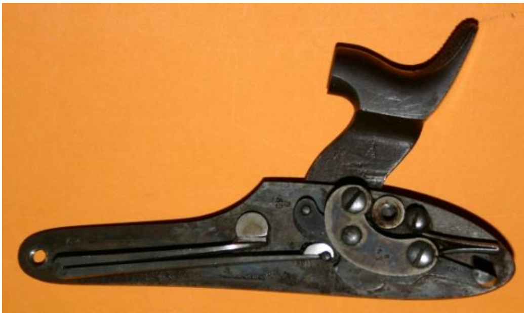
Figure 10. A Mk III Snider-Enfield percussion lock in a half cock position. 94
