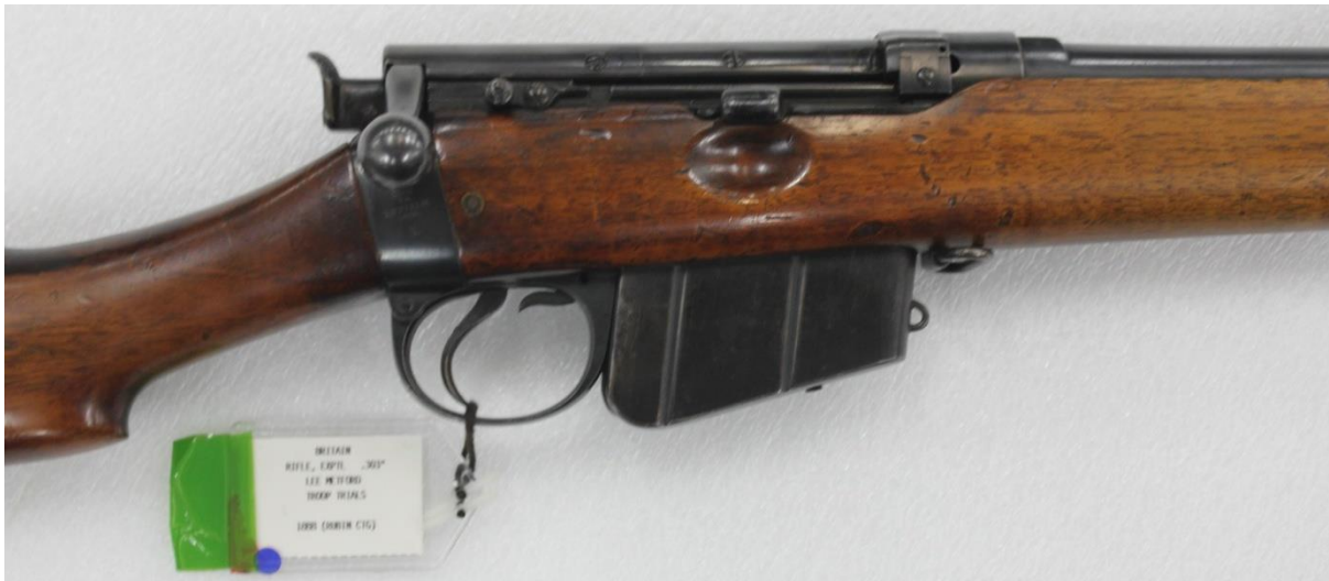
Figure 6. Rifle, Experimental, .303 Lee Metford built for troop trials. 331
