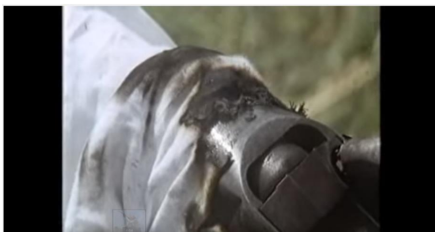
Figure 3. Captured gas leakage after firing the Sharps Carbine. 29
