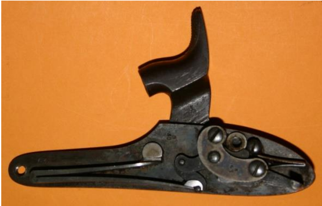
Figure 8. A Mk III Snider-Enfield percussion lock in an uncocked position.. 92
