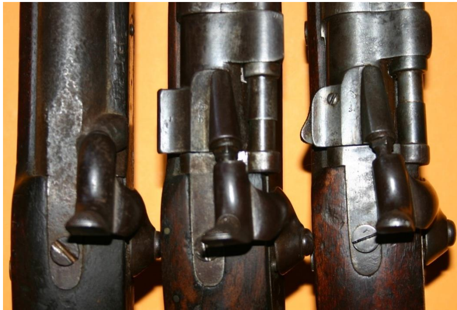
Figure 14. An overview of the Snider's breech development. Note the locking latch on the Mk III to the right. 105
