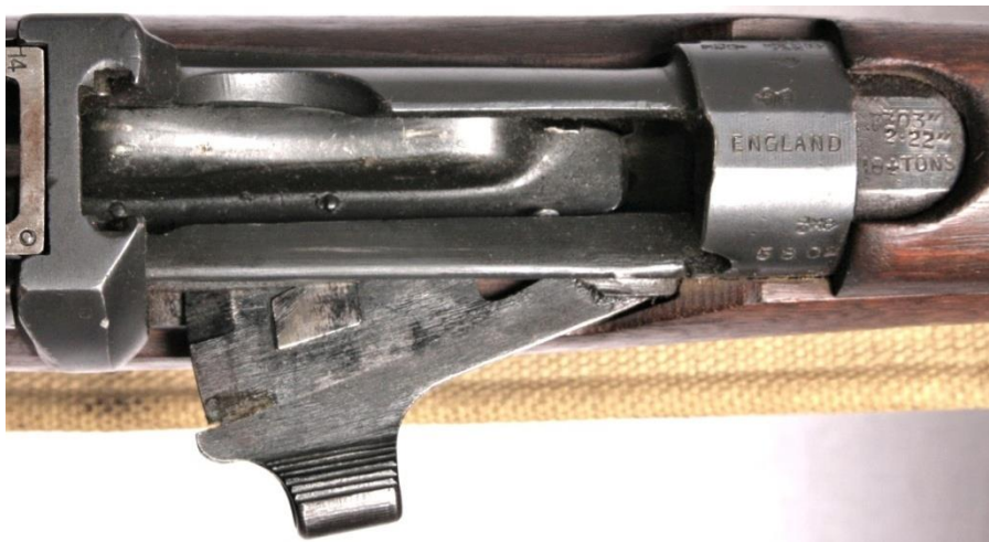
Figure 23. Magazine cut-off removed to facilitate rapid fire, the Robert W. Farris Collection. 344
