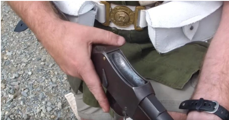
Figure 8. The lever is brought back up. Note the means of closing is different to that of opening the breech. 211
