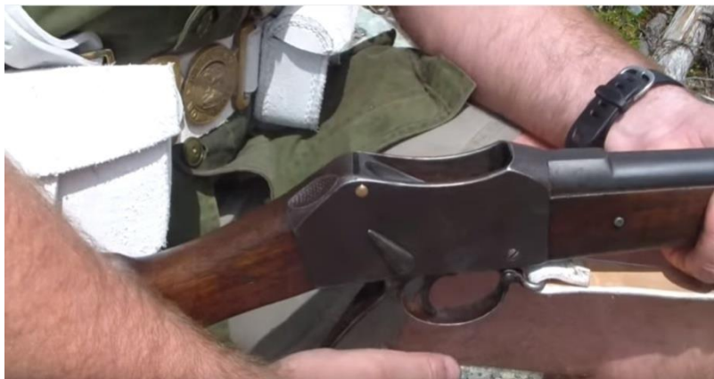
Figure 6. The breech is opened and the rifle is cocked. The cocking indicator clearly shows this as it has rotated forty-five degrees. 208
