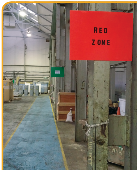
Fig. 25. Zoning (red and green) in the warehouse as a part of Project 1's future 5S plans
