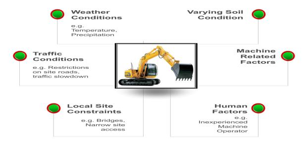
Figure 1 - Variables Affecting Earthworks Efficiency
