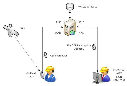
Figure 3 - System Architecture
