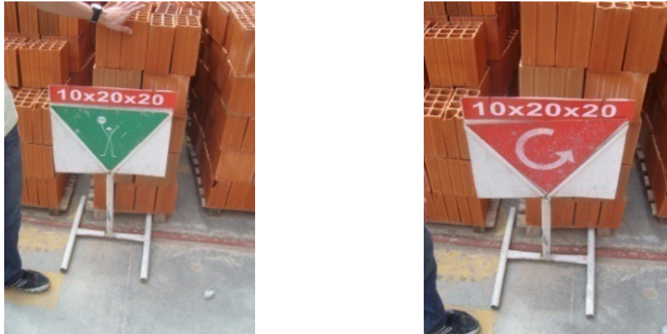
Figure 17-Pull-replenishment/production kanbans for bricks
