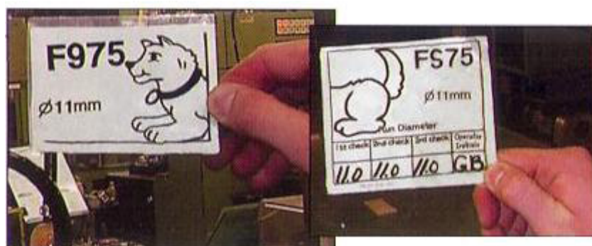
Figure 14-A card based kanban example from manufacturing (adopted from Galsworth, 2005).
