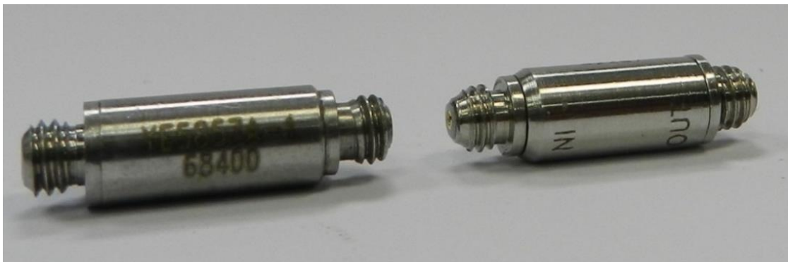
Figure 8-14: Photograph of the preamplifiers.
