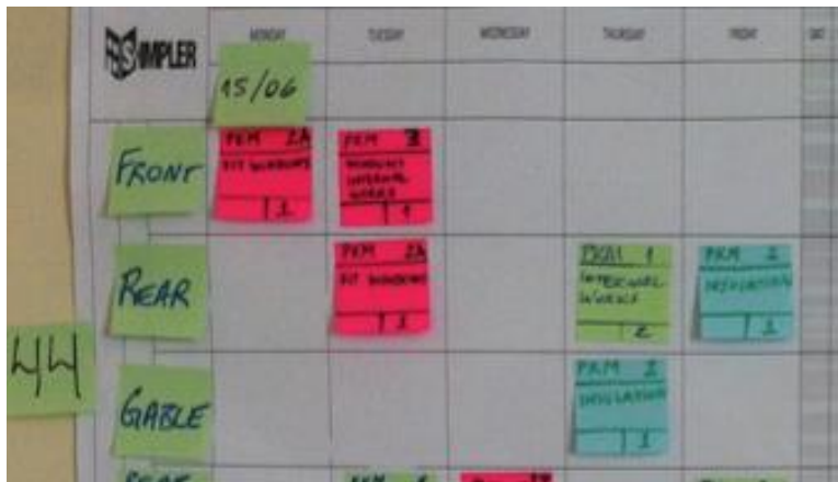
Figure 1: Post-it notes fixed on a location-based chart at the site office (master plan).
