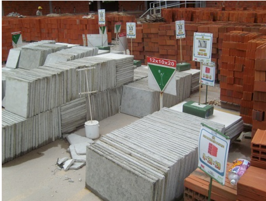
Figure 4. 5S Signs and kanban cards for material stock location standardisation and replenishment: Visual Management for process transparency and discipline
