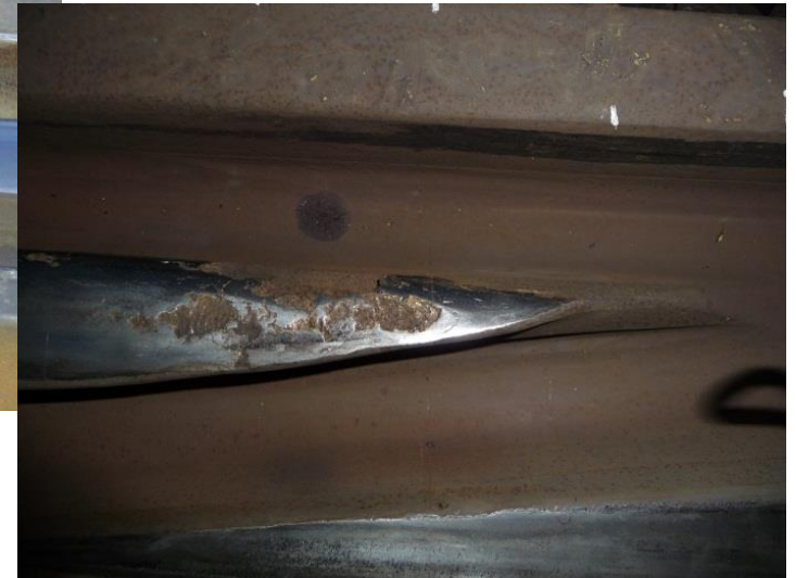
Spalling & plastic deformation of crossing nose
