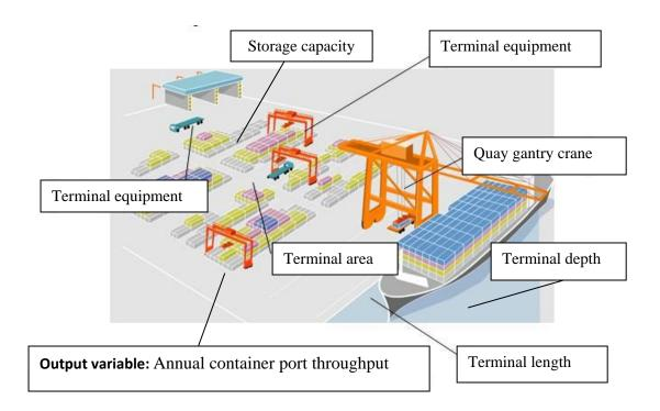
Figure 4. 6- Inputs and output variables for efficiency measurement.
