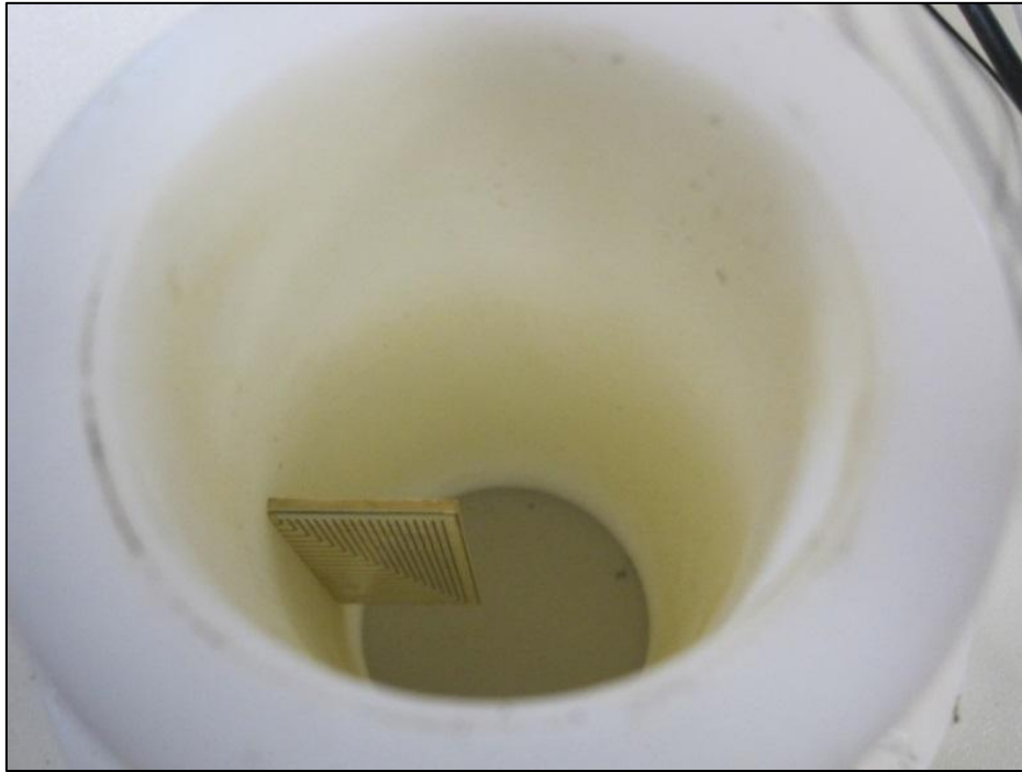
Figure 4-25: Photograph of the digital level sensor head mounted on the Venturi inlet
