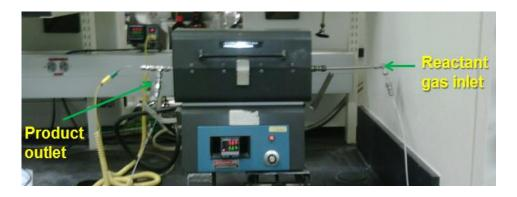
Figure 3.3. Stainless steel fixed bed and tube furnace.
