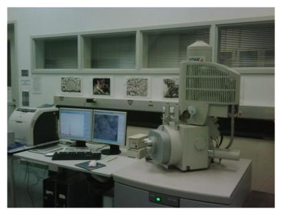
Figure 2.1. ESEM instrument FEI Quanta 400
