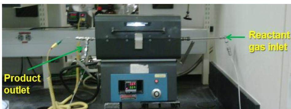
Figure 3.3. Stainless steel fixed bed and tube furnace.
