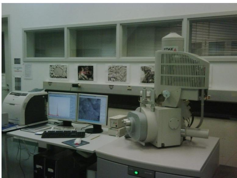
Figure 2.1. ESEM instrument FEI Quanta 400
