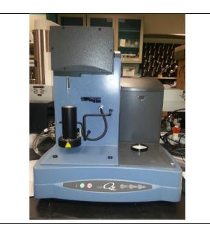
Figure 2.3. TGA instruments applied to study the carbonic deposition of selected catalyst
