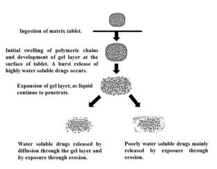
Figure 3, Release mechanism of water soluble and poorly water soluble drugs from hydrophilic matrix tablet
