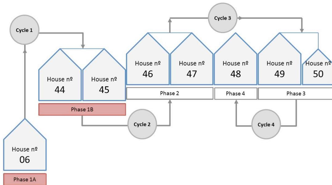
**Figure 2: Planned retrofit construction sequence**
