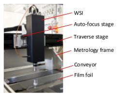
Figure 1. Opto-mechanical system on film re-winder stand
