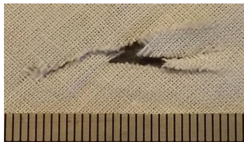
Figure 74: After weathering – bias stab cut 27mm in length (single edged blade).
