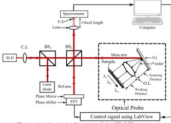
Figure 1: schematic diagram of the SDSCI system
