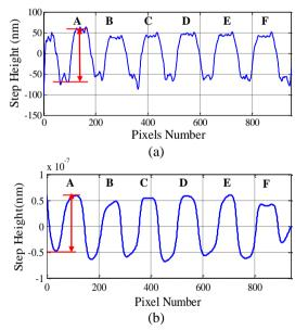
Figure 3 A measured surface profile on the waffle plate using SDSCI system using (a) PSI; (b) FTP.
