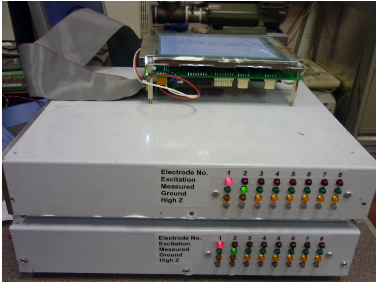
Figure 5.2 Electrodes selection circuits integrated with VM-1 microcontroller
