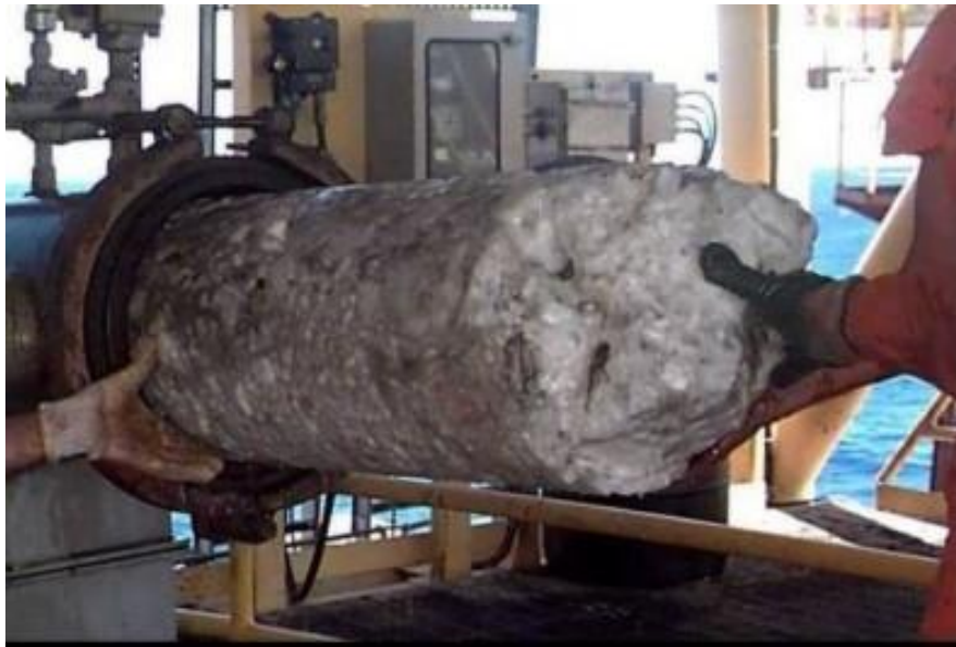
Figure 1.4 A large gas hydrate plug formed in a subsea hydrocarbon pipeline.[26]
