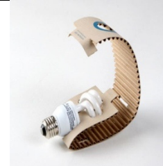
Figure 2.17. Singleface corrugated board
