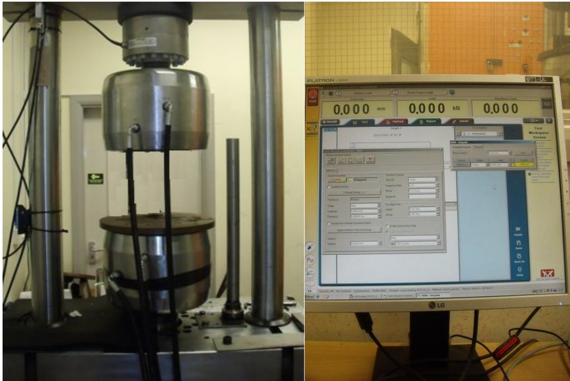
**Figure 7-13: Fatigue testing machine**
