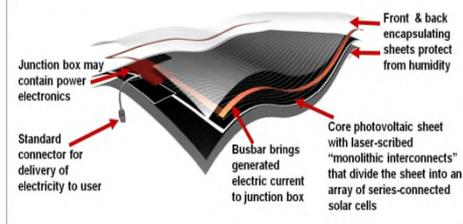
Front & back encapsulating sheets protect from humidity
