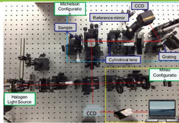
Experimental setup of the SRWLI system
