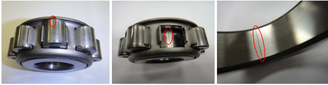
(a) 30% roller fault (b) 60% inner race fault (c) 100% outer race fault
