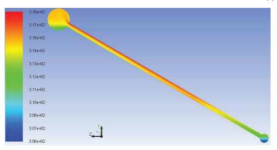
Figure 3 Temperature variations within the thermo-syphon after 1 hour of operation
