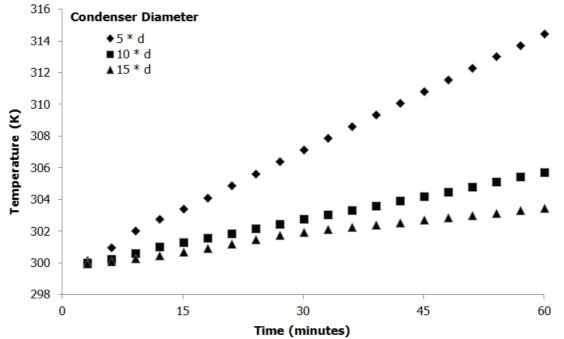
Figure 5. Temperature variations within the various condensers for 1 hour of operation
