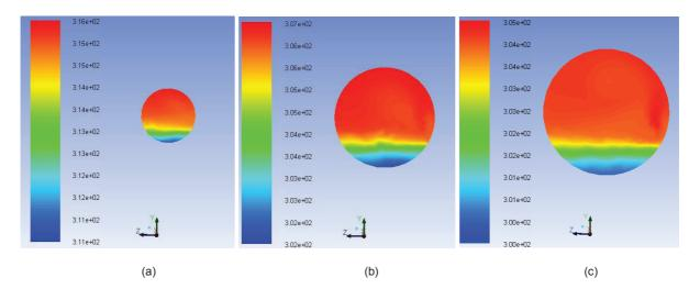
Figure 4 Temperature variations within various condensers after 1 hour of operation (a) Condenser diameter = 5 \* d (b) Condenser diameter = 10 \* d and (c) Condenser diameter = 15 \* d
