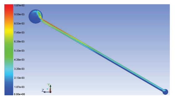
Figure 2. Velocity variations within the thermo-syphon after 1 hour of operation
